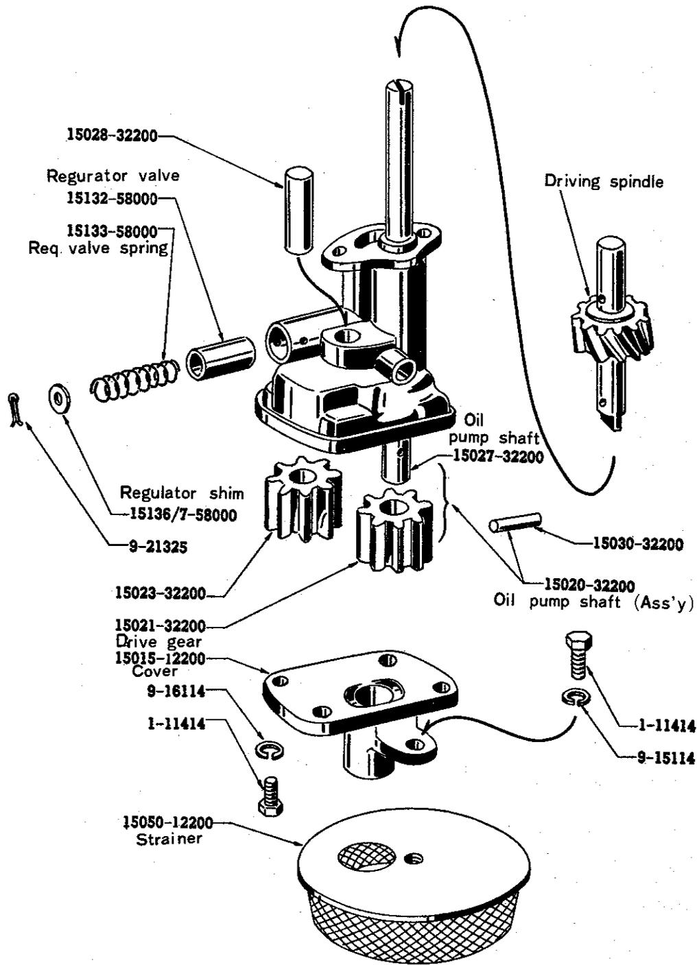
Fig. 6 Oil pump & strainer assembly
