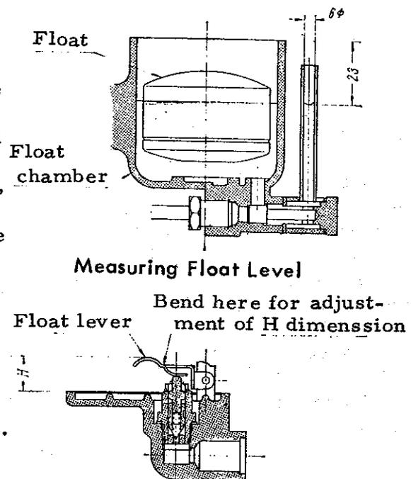
Fig. 5 Adjusting Float Level
