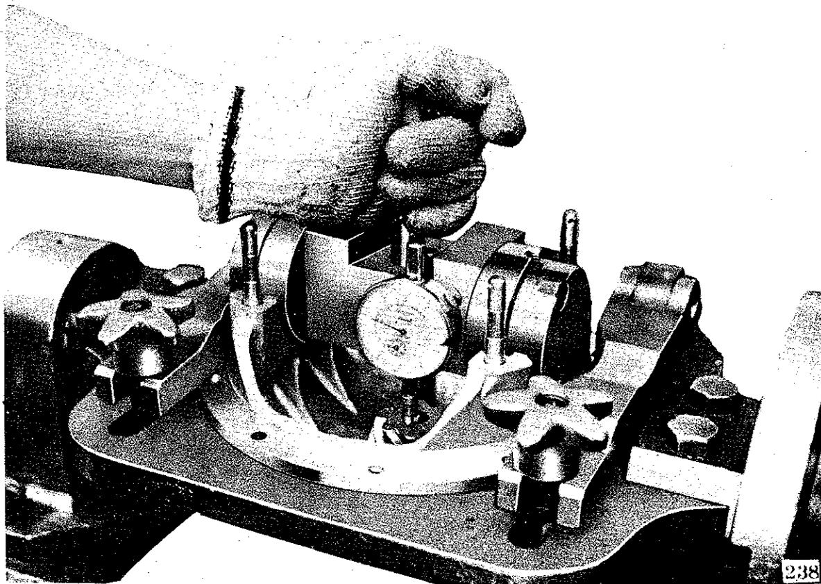
Fig. 9 Adjustment of Pinion Height
