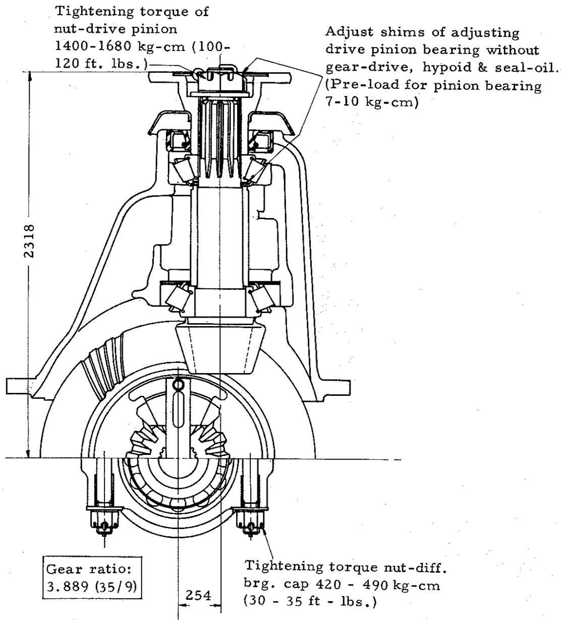
Fig. 3 Section of differential case
