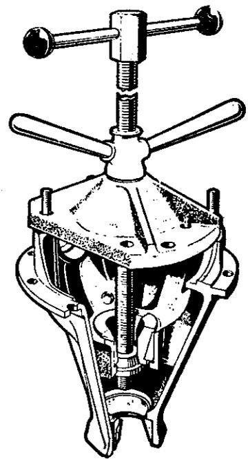
Fig. 4 Drive pinion front and rear bearing outer race replacer
