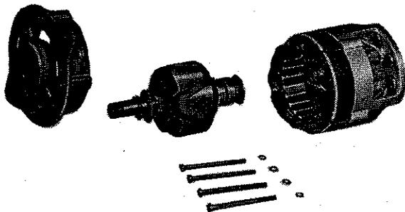
Remove the thru bolt (23131-12210) tightening bolt front cover (23118-12210) and rear cover (23127-12211), pull off the front cover and rotor (23108-12210). Use a hammer of wood or plastic if necessary.
