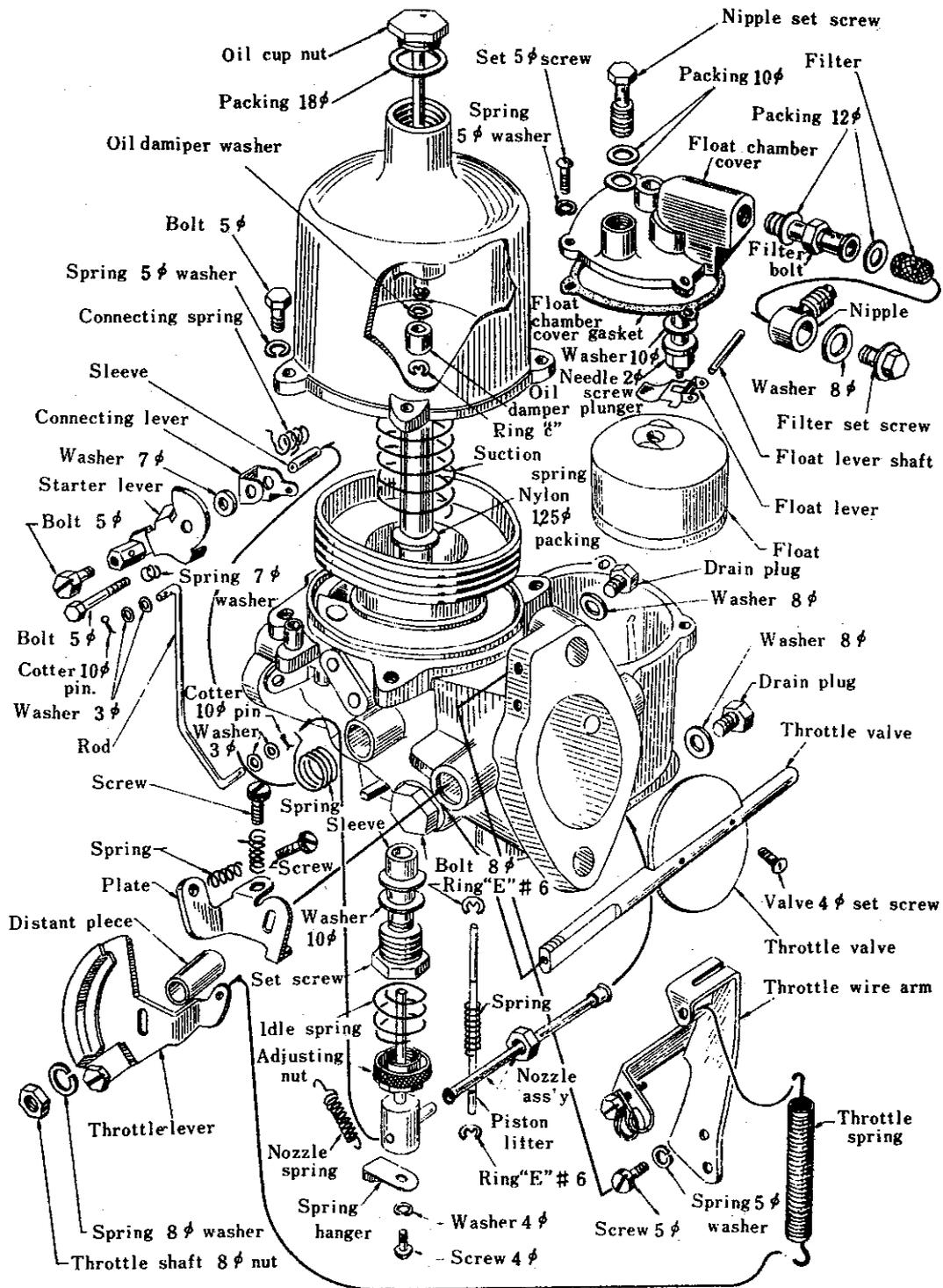
Fig.9 Key to the Carburetor Components
