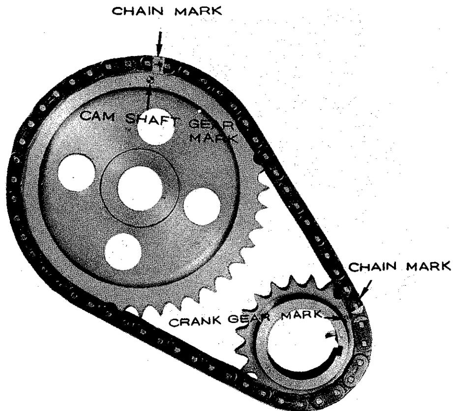
Fig. 2 Position of refitting gears with the chain
