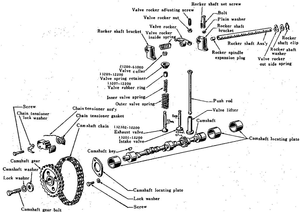
Fig. 10 Camshaft & valve gear
