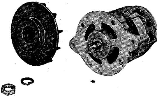
Remove the hex. nut (23153-12210) of pulley (23151-12210) and pull off the pulley and the half-moon key (23195-12210). Be careful not to injure the fan when the nut is removed.
