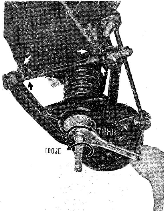
Fig. 7. Refitting the coil spring
