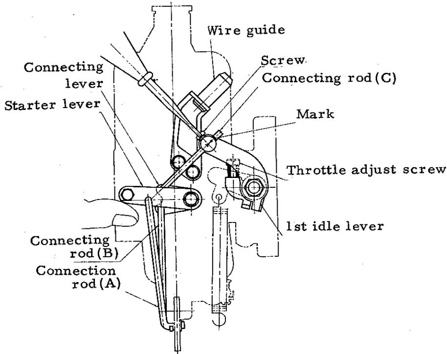
**Fig. 6 Adjustment for Opening degree at connecting**
