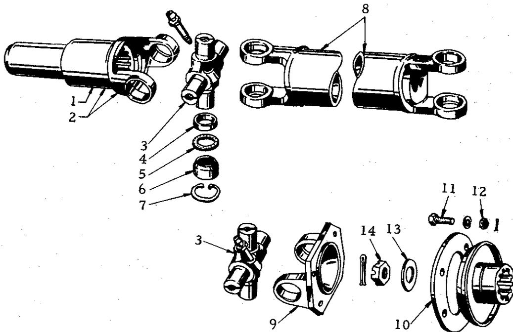
Fig. 1 Propeller shaft & joint
