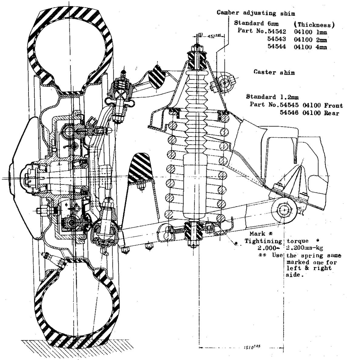
Fig. 3 Section of front suspension
