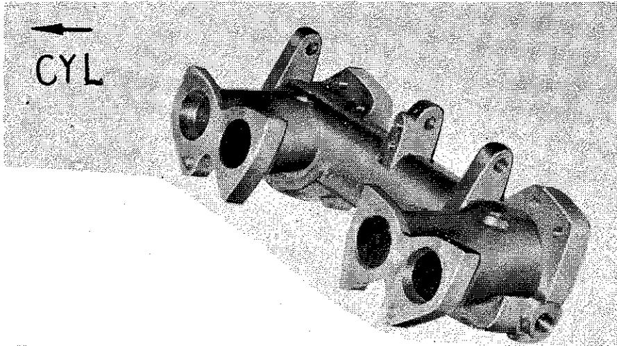
Fig. 3 Intake manifold
