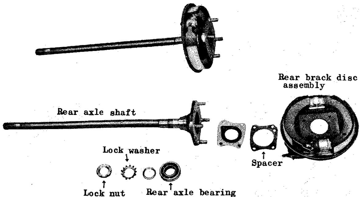
Fig. 2 Rear axle shaft & brake disc assembly
