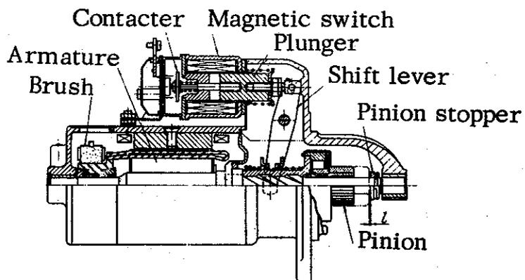
Fig. 1 Sectional view of magnetic shift type
