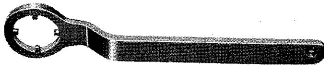
Rear axle shaft bearing lock
