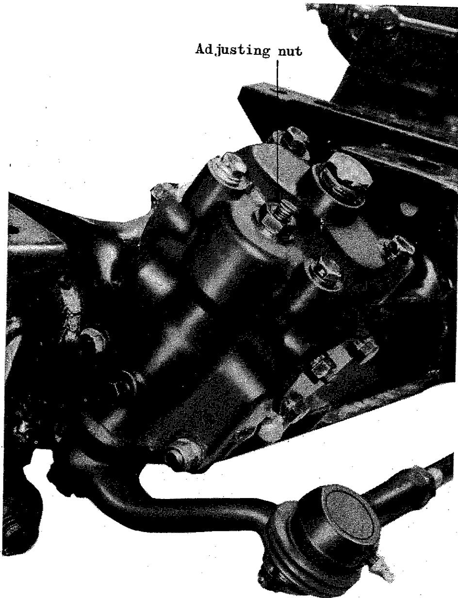
Fig. 1 Steering gear box
