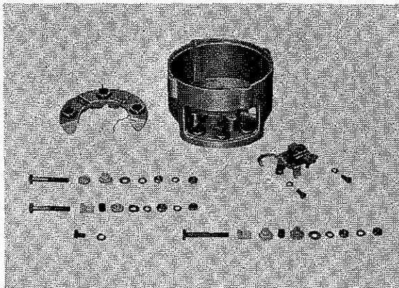
Remove the diode set and brush holder (23133-12210) from the rear cover, when be careful not to lose small parts such as screws, washers and bushings.
