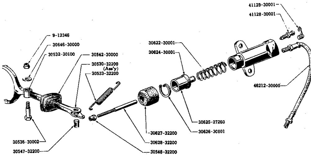
Fig. 2 Clutch operating
